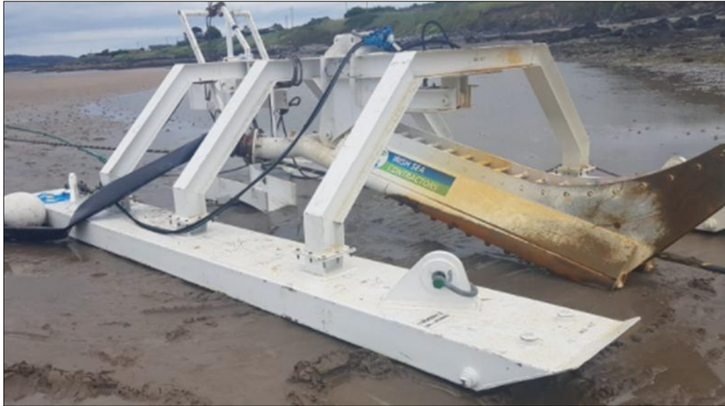
Figure 6. Example Jetting Sled as Option for Easing Cable Recovery
